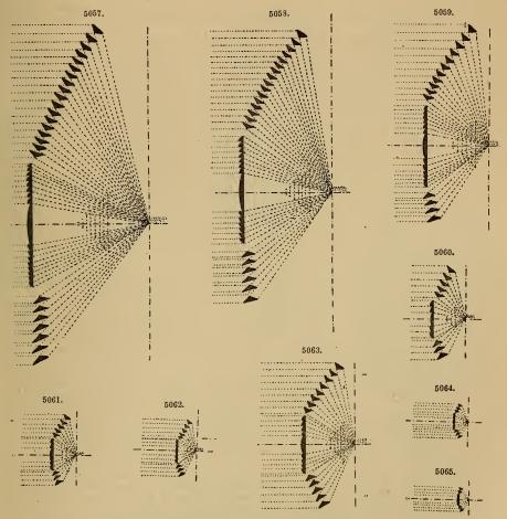
The Fourth Order, being the largest of the harbour lights, has an internal diameter of 0.5 mètre = 19.685 in., and a height of glass of 0.739 mètre = 29.112 in., Fig. 5060. The Fifth Order, Fig. 5061, has an internal diameter of 0.375 mètre = 14.764 in., all the dimen-
